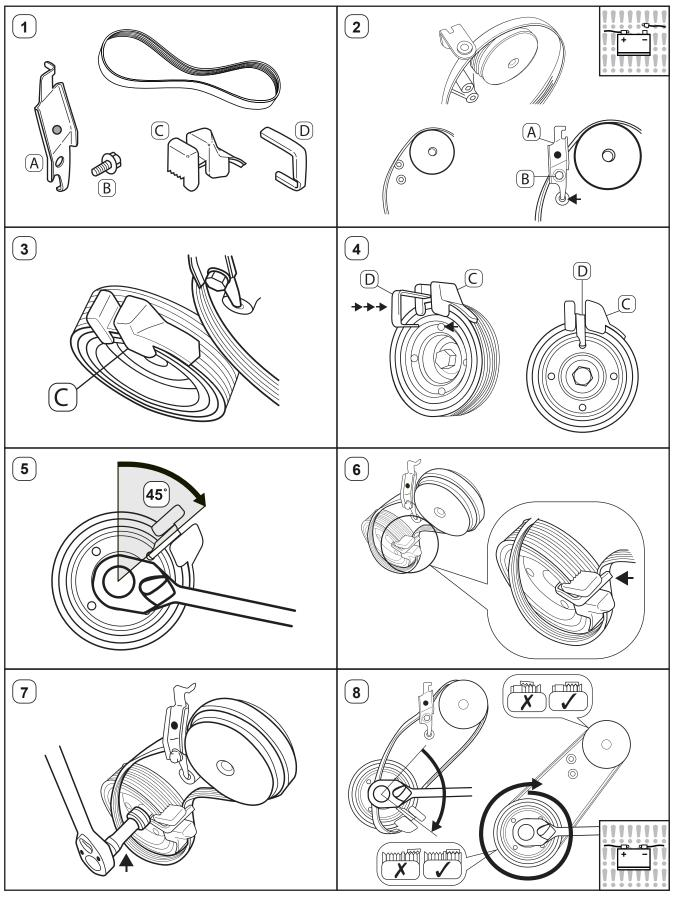
Storing product above 100°F/38°C could result in belt shrinking, affecting installation
