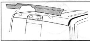
**STEP 1:** Test fit part on vehicle prior to install. Clean the areas on the roof where the cab spoiler will contact the sheet metal using soap and water. A secondary cleaning of isopropyl alcohol can be used, but is not required.
