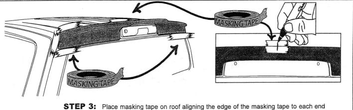
on the cab spoiler. Place masking tape centrally on the roof sheet metal and cab spoiler, mark line with a non-permanent pen to assist in positioning.
