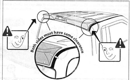
**STEP 2:** Align cab spoiler centrally on the roof, ensuring equal spacing around the Center High Mount Stop Light and at both ends of the spoiler to the roof weather-strip channel.
