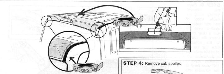
**STEP 3:** Place masking tape on roof aligning the edge of the masking tape to each end on the cab spoiler. Place masking tape centrally on the roof sheet metal and cab spoiler, mark line with a non-permanent pen to assist in positioning.
