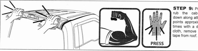
STEP 9: Press and rub the cab spoiler down along attachment points approximately 5 times with a dry clean cloth, remove masking
