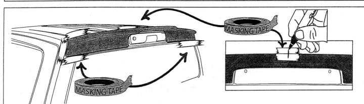
**STEP 3:** Place masking tape on roof aligning the edge of the masking tape to each end on the cab spoiler. Place masking tape centrally on the roof sheet metal and cab spoiler, mark line with a non-permanent pen to assist in positioning.
