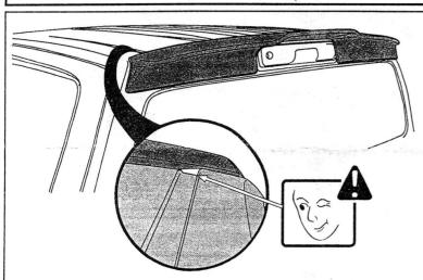
**STEP 2:** Align cab spoiler centrally on the roof, ensuring equal spacing around the Center High Mount Stop Light and at both ends of the spoiler to the roof weather-strip channel.
