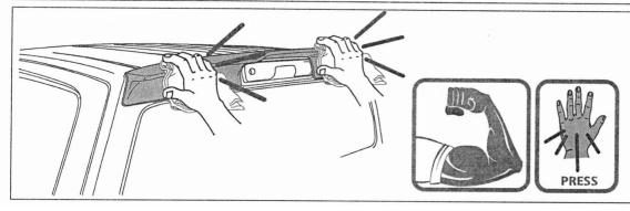
**STEP 8:** Press and rub the cab spoiler down along attachment points approximately 5 times with a dry clean cloth, remove masking tape from roof.
