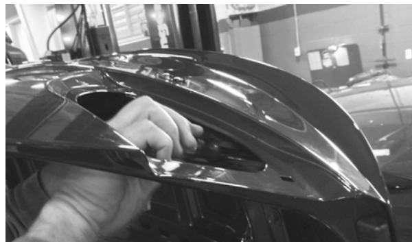
Screwing Spoiler into Deck Lid >
