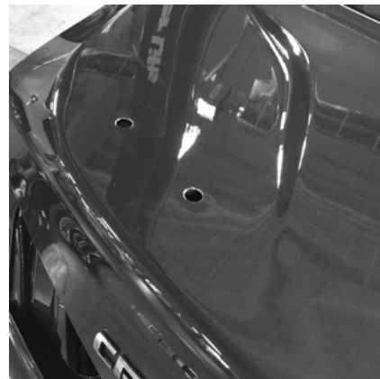
2 of 4 Drilled Spoiler Holes
