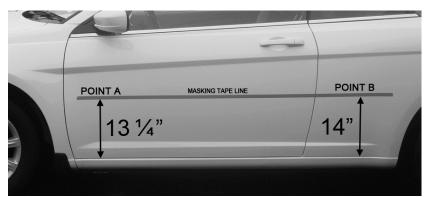
Measure up from bottom of door in front, continue to follow door line to the rear of the vehicle and measure up.
