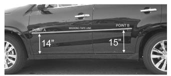
If model does NOT have cladding, measure up from bottom of doors.
