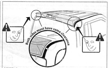
**STEP 2:** Align cab spoiler centrally on the roof, ensuring equal spacing around the Center High Mount Stop Light and at both ends of the spoiler to the roof weather-strip channel.
