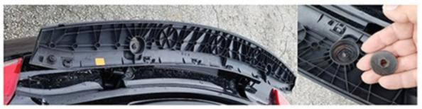
Once top cover is removed, remove the 2 nuts holding the bottom base cover. Remove cover, save the 2 nuts to attach wing brackets with.
