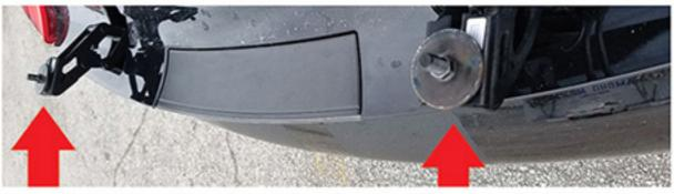
If the height of the spoiler need to be adjusted, these are the Nuts that can be adjusted to correct the height.
