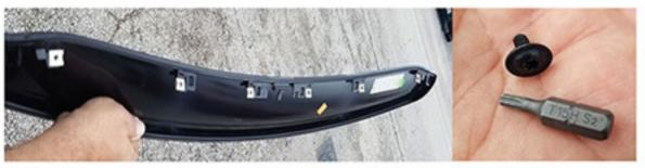
Once raised – Remove screws with T15 Torx Tool, along the front edge and remove spoiler cover.
