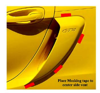
2. Before removing Red tape Backing, Center Side Vents on car, then place masking tape to outline correct fit. Apply 3M Adhesion Promoter (Included) to Body Edge where Double side tape will adhere to.
