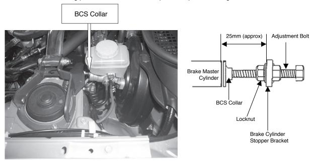
Note: Do not over tighten the Brake Cylinder Stopper Adjustment Bolt. Doing so may cause permanent damage to and components around the brake master cylinder.
