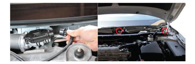
4.) Disconnect the main wiper motor harness. Remove four plastic fasteners by pinching the tabs underneath with needle nose pliers and set the wiring loom aside.
