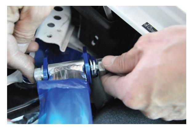
8.) Install the main bar with the washers and crush washer in this order. Hand tighten both ends, then torque down with a 17mm wrench and hex allen head driver.
