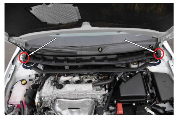
3.) Remove two plastic clips located on the left and right corners of the plastic cowl. Pop in the center dowel first to easily pull off the clip. Carefully remove entire plastic cowl tray from vehicle, exposing the wiper motor assembly (There are bumps in the plastic indicating the locations of the clips).
