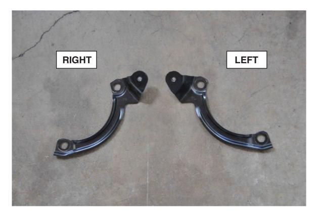
7.) Remove and discard the factory apron extensions located on the top of both strut towers. These are held down by 14mm nuts on each side. Remove the third nut on the strut tower on both sides.
