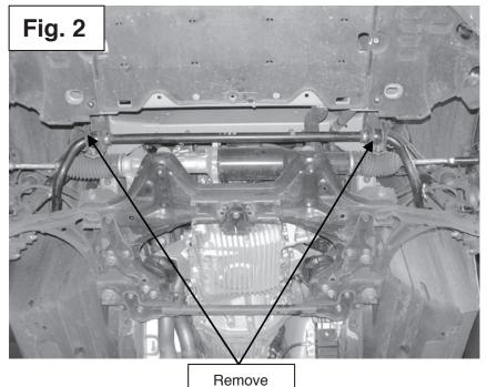
4.) Install the sway bar in the reverse order that it was taken off or refer to the factory service manual for step by step instructions as well as the correct torque specs.
