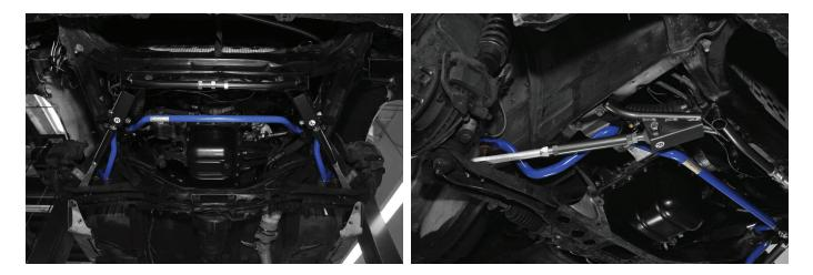
\*Periodically inspect and retorque all nuts and bolts after vehicle operation.
