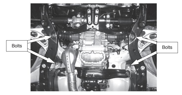
3.) Install the Cusco lower arm bar in the position shown by reusing the removed bolts in step 2. Torque according to factory service manual specifications.
