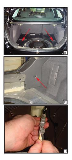
6. Route the T-Connector end with the green wire out from behind the felt trunk liner across to the passenger side behind the removed rear scuff panel. Repeat Step 2 on the passenger side using the T-Connector end with the green wire.
