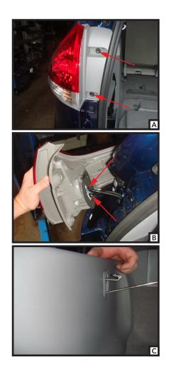
6. Route the black power wire from the battery as shown on the CME-PCL-INS sheet included. In the rear of the vehicle route the black wire up thru the opening under the drivers side taillight.
