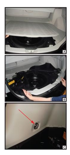
5. Locate a suitable grounding point near the connector such as the vehicle's frame or cross member. Drill a 3/32" hole and secure white wire using eyelet and screw provided.
