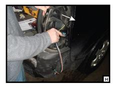
4. From the passengers's side taillight pocket route the T-connector end with the yellow wire ,the 4-flat, and the black converter box down through the opening made in step 2 and 3. GHT From underneath the vehicle route both wires reward to the backside of the bumper fascia. Route the 4-flat to the center of the vehicle. Route the yellow wire to the driver's side and up to the drivers side taillight.
