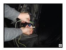
1. Open the hatch and remove both taillight assemblies by removing two Torx-15 head screws on each. A B Behind the taillight assemblies locate the vehicles taillight wiring harness the harness will have connectors similar to those on the T-connector harness. Separate the connectors being sure not to damage the locking tabs. C Set taillight assemblies aside.
