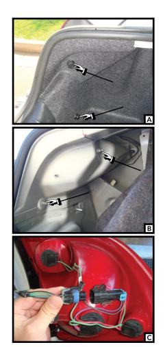
2. On the passenger's side locate a suitable grounding point near the connector such as an existing screw with nut in the vehicle's frame or drill a 3/32" hole and secure white wire using eyelet and screw provided.
