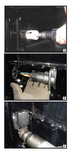
5. Using a hole saw, drill a 2 1/8" hole in the desired location in the sidewall.
