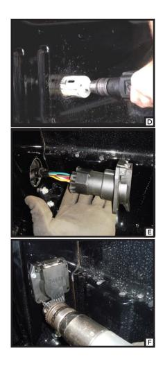
5. Using a hole saw, drill a 2 1/8" hole in the desired location in the sidewall. D
