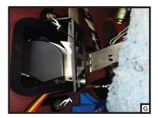
1. Open the rear hatch and remove two 10 mm bolts on each taillight assembly. A Pull out on the taillight assemblies being sure not to damage the alignment tabs. Behind the taillights locate the vehicles taillight wiring harness it will have connectors similar to those on the T-connector harness. Separate the connectors being sure not to damage the allignment tabs, set taillights aside.
