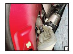
4. On the drivers side route the T-connector end with the yellow wire behind seatbelt bracket and out through the grommet and insert in-between the separated connectors make sure the connectors are fully inserted with locking tabs in place.
