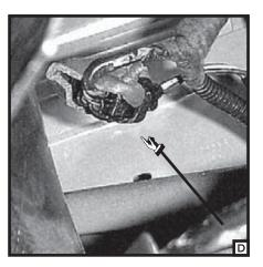
6. Bundle and secure wires to the vehicle's cross member using the cable ties provided. Route the 4-Flat to the center of the vehicle's cross member using cable ties provided. Reinstall protective covers removed in step 1.
