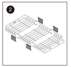
Secure the extension into the 2 halves of the basket. Attach the side fairing brackets and secure with the machine screws provided 2.
