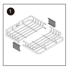
Remove protective plastic end caps. Remove the 4 machine screws and side fairing brackets from the basket and separate into two halves using the wrench provided.
