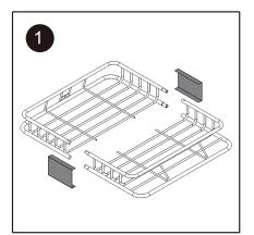
Remove protective plastic end caps. Slide the front and rear basket together. Attach the side and rear small fairings as shown in diagram 1. Secure the assembly with machine screws 8. Position basket on the roof bars of your vehicle.
