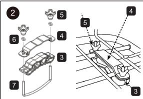
Now snap the saddle 3 into the basket. The saddle must sit on the cross bar. Secure it with the bracket top plate 4, knobs 5, washers 6 and U bolts 7.
