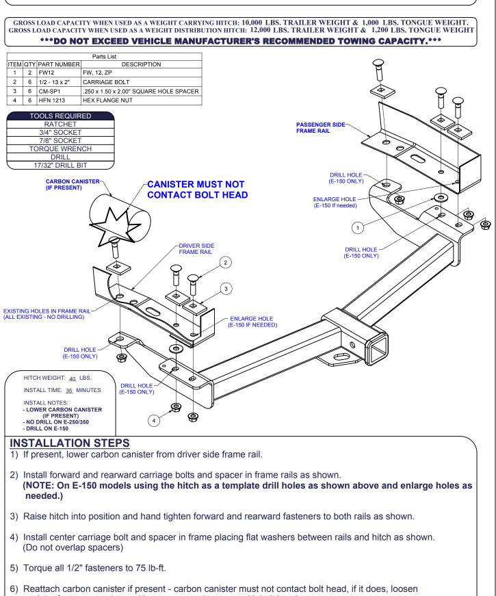
canister fasteners and reposition to ensure clearance with bolt heads. PERIODICALLY CHECK THIS RECEIVER HITCH TO ENSURE THAT ALL FASTENERS ARE TIGHT AND THAT ALL STRUCTURAL COMPONENTS ARE SOUND.
