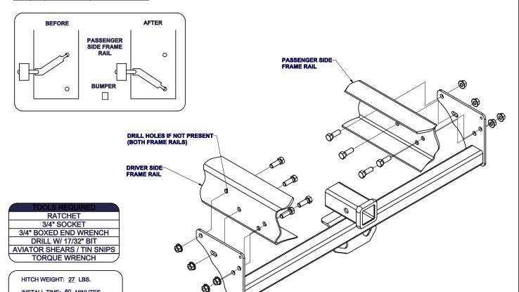
MAY REQUIRE DRILLING - EXHAUST BRACKET RELOCATION
