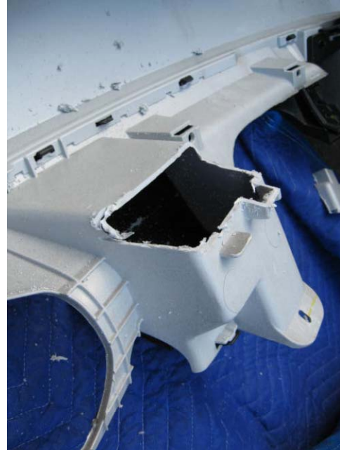
USING A ROTARY OR EQUIVALENT CUTTING TOOL, TRIM BUMPER FASCIA AS SHOWN TO THE RIGHT.
