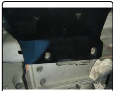
4. Secure the passenger side using the existing weld nuts, the M12 hex head bolts and the 1/2" conical toothed washers provided.
