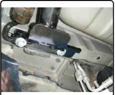
6. Torque all M12 fasteners to 60 ft. lbs. Raise exhaust back into position.
