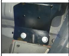
5. Sandwitch the driver side with the muffler hanger bracket and secure using the M12 hex head bolts and the 1/2" conical toothed washers provided.
