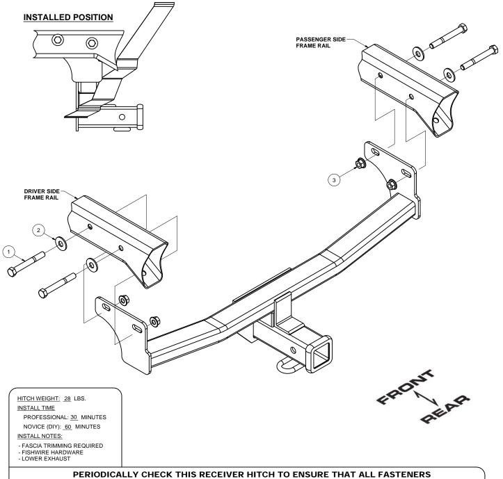
PERIODICALLY CHECK THIS RECEIVER HITCH TO ENSURE THAT ALL FASTENERS
