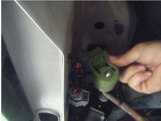
EXHAUST HANGER REMOVAL
