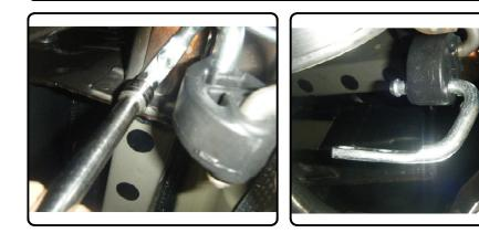
4) Raise the hitch into position and install (3) 10mm bolts and conical toothed washers per side into the existing weldnuts in the frame. If the vehicle is all wheel drive then reinstall the sway bar brackets using CM-SP50 spacer blocks and the existing nuts on the lower mounts.
