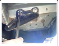
2) Lower rear most exhaust isolator for ease of installation.
