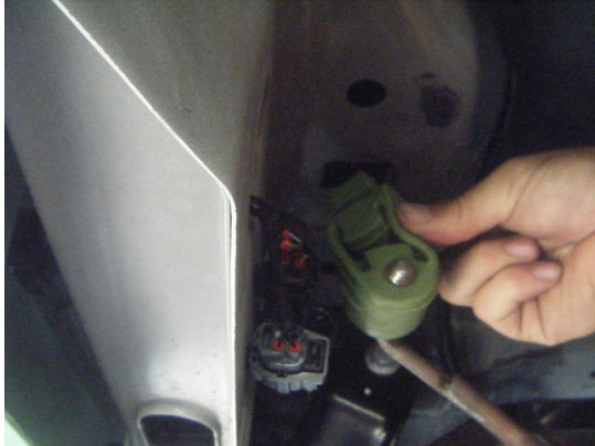
EXHAUST HANGER REMOVAL
