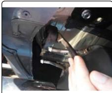
2. Remove heat shield(s) by removing four fasteners per shield. Save fasteners for reinstallation.
