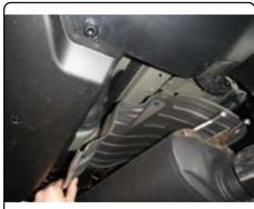
3. Fishwire 7/16"-14 x 1 1/4" carriage bolts with CM-SP2 spacers into poistion through access holes in both frame rails, as shown on page 1. See FISHWIRE TECHNIQUE DIAGRAM below. **NOTE:** Leave fishwires attached to prevent loss of hardware inside of frame rail.
