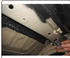
4. Insert 3/8" U-bolt through tow hook, as shown.
