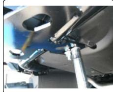
7. Trim heat shield(s) around hitch. Reinstall heat shield(s) with hardware removed in Step 2. **NOTE:** One fastener per shield will not be reinstalled. See HEAT SHIELD TRIMMING DIAGRAM below.
