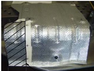
3-1/2" AREA TO TRIM HEAT SHIELD TRIMMING DIAGRAM
