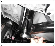
6. Reinstall rubber isolator (if it was removed in step 1).
