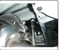
2. Remove existing bolts from tow loop. Return tow loop and bolts to owner. **NOTE:** Access bolts through tow loop cut out in the underbody panel on standard Prius models.
