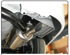
5. Torque all 12mm fasteners to 72 ft-lbs.
