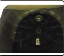
11) Adjust large spacers, trunk strap and hitch to be square with vehicle. Torque all 7/16" fasteners to 50 lb-ft, all 1/2" fasteners to 75 1b-ft.
