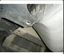
5) Remove material between adjacent holes in frame rail using metal shears or die grinder. Enlarge opening to allow the head of a 7/16" carriage bolt to pass through. Repeat for other side of vehicle.
