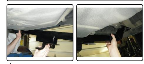
8) Being careful not to push bolts back into frame, lift hitch into position. Install flange nuts, finger tighten.
