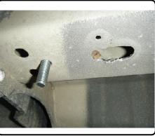
7) Raise hitch into position while holding plastic fascia support fingers back to allow hitch main body to fit up into cavity behind bumper.
