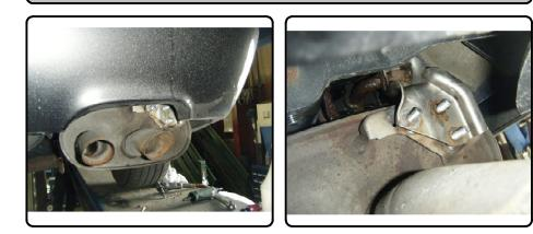
4) Remove plastic rivets from supports on bottom edge of bumper fascia. Rivets are released by first pulling out center post approximately 1/4". Rivet can then be pushed out by hand.
