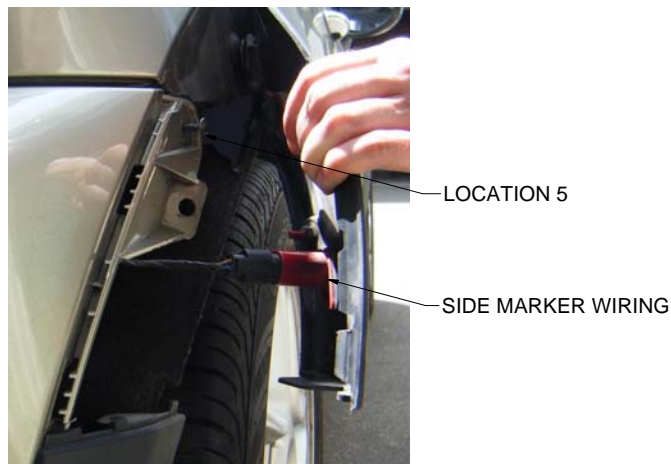
Photo 4: Fastener C behind wheel moulding.
