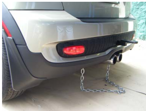
Photo 13: Hitch shown installed with safety chains
