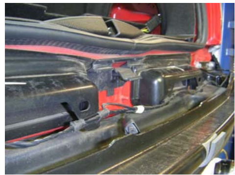
Photo 12: Center alignment feature.
