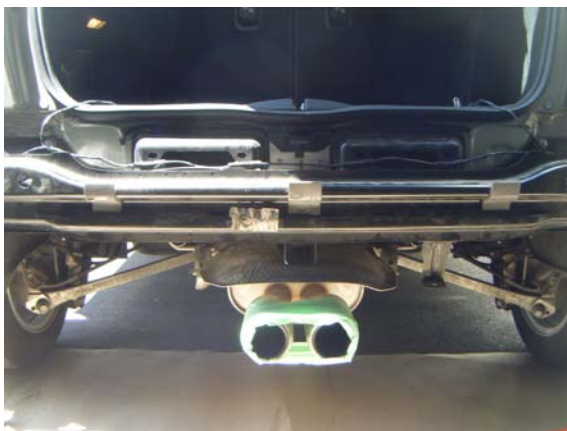
Photo 9: Hitch and bumper beam installed
