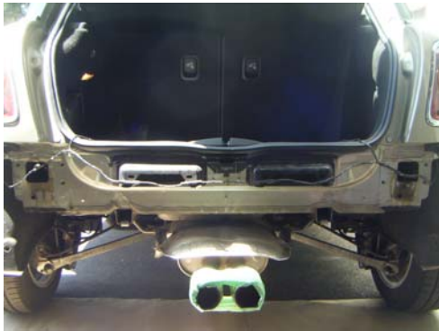
Photo 7: Bumper beam removed.
