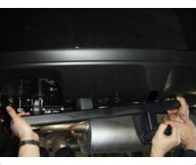
4. Remove forward most rubber plug from each frame rail.
