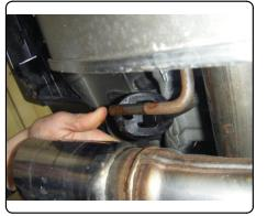
2. Remove (2) brackets which hold fascia to vehicle. These will be reinstalled in step 8.
