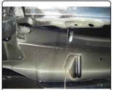
7. Thread fishwires through appropriate mounting holes on hitch and raise hitch into position.
