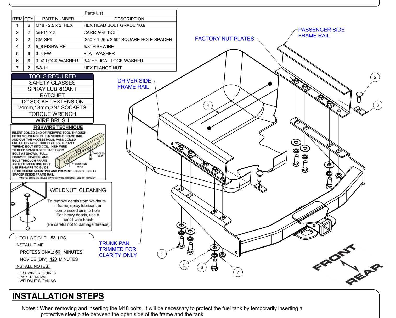
Remove OEM hitch prior to CURT hitch install. OEM hitch is held on by (6) M18 bolts and (2) M18 shear
