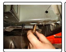
9. Raise hitch into position over the heat shield and loosely fasten the side plates with 3/8" and 7/16" flange nuts on both sides. Loosely fasten M8 hardware in the two forwardmost weldnuts on each frame rail and the muffler bracket.
