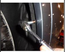
3. If applicable, disconnect the backup sensors attached to the rear bumper. Remove the rear bumper cover.
