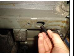
7. Fishwire 7/16-20 x 1 1/2" carriage bolts and SP2 spacers through access hole "A" to hole "B" located on the outside of each frame rail.
