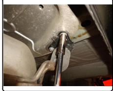
5. Cut a notch in the heat shield to clear the middle hole on the driver side frame rail using shears.
