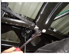
2.) Remove (4) bolts securing the factory crossmember or hitch to the frame rail with a 21mm socket. Set hardware aside for reuse during CURT hitch installation. Note: The bumper shares the same mounting points and should be supported from underneath.
