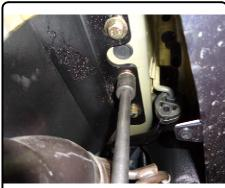
4.) Torque all M12 hardware to 86 ft-lb. Reattach all exhaust hangers.
