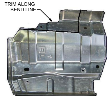
HEAT SHIELD TRIM DIAGRAM
