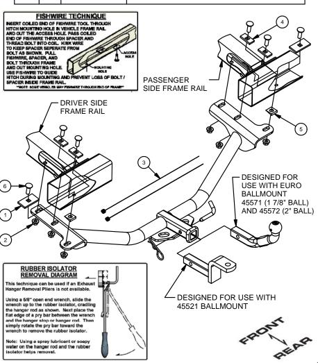
1.) Lower exhaust by removing rubber isolators (3 each side) as shown.
