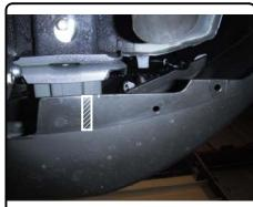
4) Thread the fishwires though the corresponding holes in the hitch and raise into position. Remove fishwires and loosely install the (4) supplied hex flange nuts.
