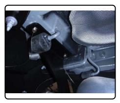
5) Raise the exhaust back into position, one side at a time, if lowered and reinstall isolators.
