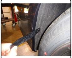
2. Remove (1) screw hidden behind the wheel well at the top of the facia. Remove the plastic clip by prying it out with a flat head screw driver.
