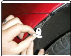
3. Remove small plastic panel between tail light and trunk opening. Remove exposed screw.
